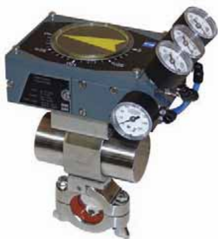
B5102 butterfly valve, silicone seat, stainless steel horizontal actuator, double acting, NEMA 4/4X 3-15PSI pneumatic positioner
