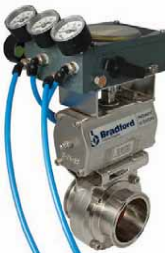
B5101 butterfly valve, silicone seat, clamp x clamp, stainless steel rack and pinion actuator, spring return, NEMA 4/4X 3-15PSI pneumatic positioner
