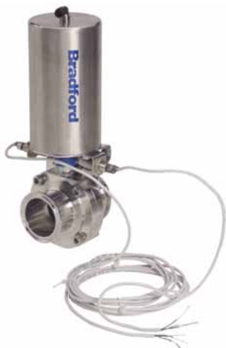
B5101 butterfly valve, silicone seat, clamp x clamp, stainless steel vertical canister, spring return, normally closed, (2) 10-30VDC proximity sensors
