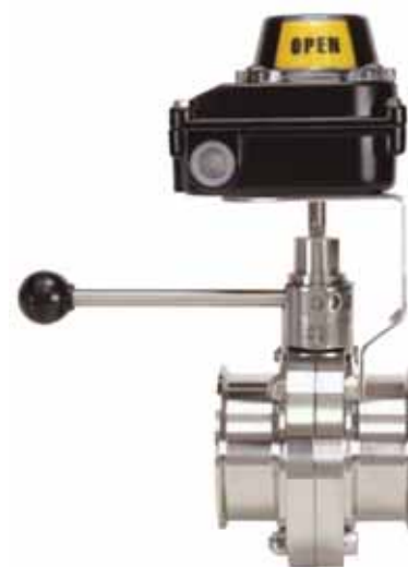
B5101 butterfly valve, EPDM seat, clamp x clamp, standard 4-position handle with a NEMA 4 SPDT limit switch with 2 mechanical switches
